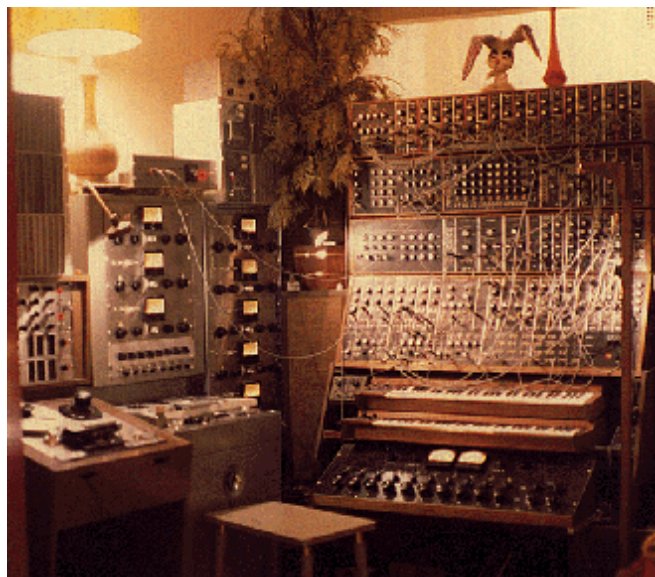
Figure 1.7. A Moog analog subtractive synthesizer.
